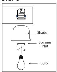
Remove spinner nut from socket. Position shade on lamp and secure with spinner nut.
