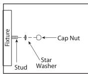
Tuck electrical wires into electrical box and position fixture over studs on mounting bracket assembly. Secure fixture in place with star washers and cap nuts.
